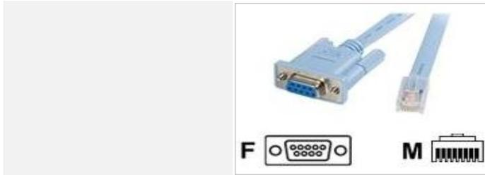
**Step 2:** Connect the F port of the serial cable to the COM port of PC.
