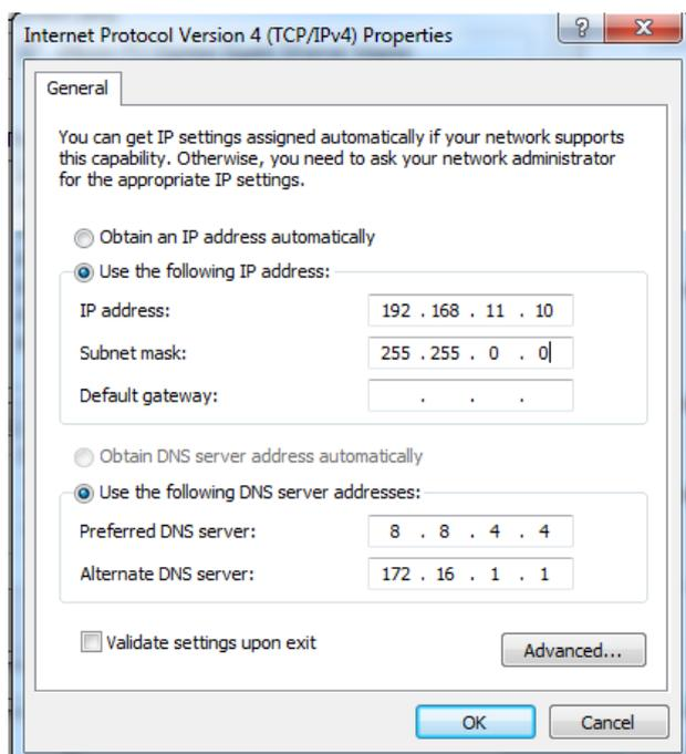
Check the connectivity between the PC and the gateway. Click **Start** → **Run** of PC and enter cmd to execute 'ping 192.168.11.1' to check whether the IP address of the DAG2500-72S gateway runs normally.
