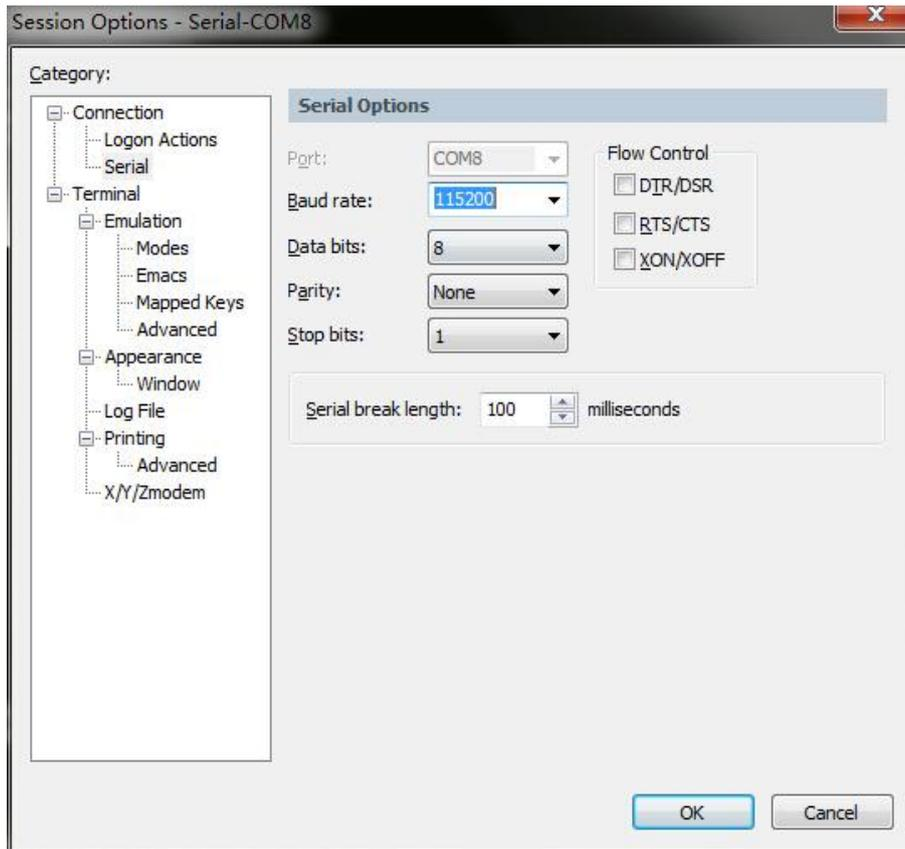
3. Click **OK**, and then enter 'ifconfig', and the IP address of GE1 or GE0 of MTG2000 will be displayed.
