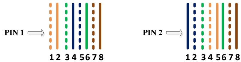
3. Put the lines into two pins of RJ-48 joint according to the abovementioned sequence of the lines.
