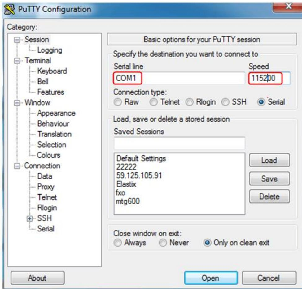
After finishing the above configuration, click the **Open** button to enter the following interface.
